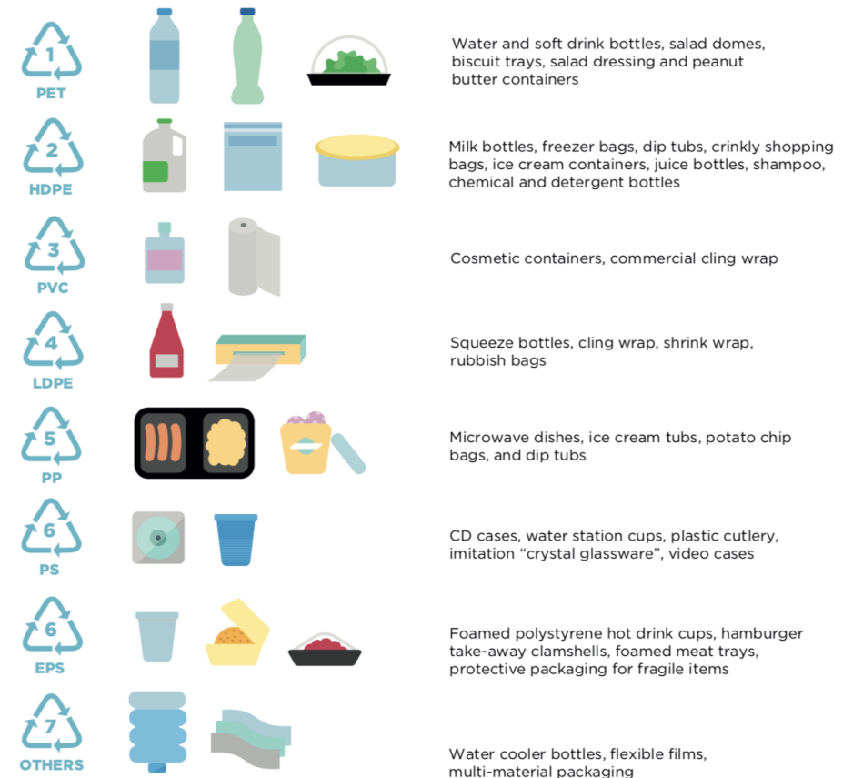
Figure 2: Main Plastic Resin Types and Their Applications in Packaging
